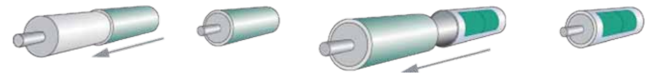
1. Bridge sleeve mounting on shaft 2. Bridge in normal position 3. Top sleeve mounting 4. Utilization in printing process
