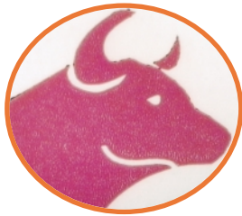
Initial print quality with R/bak SA 2320 tape.
