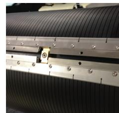
The automatic clamp system makes plate loading very easy.
